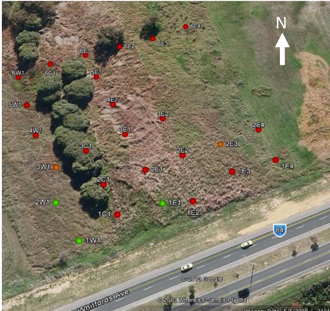
Figure 2. Illustration of the sites where sediment samples were collected to a depth of 1.5 m. Green indicates sites where soil types throughout the profile did not exceed the action criteria, amber indicates sites where soil types throughout the profile were equal to the action criteria and red indicates sites where soil types throughout the profile exceeded the action criteria. The action criteria were based on SPOCAS and SCR results.
