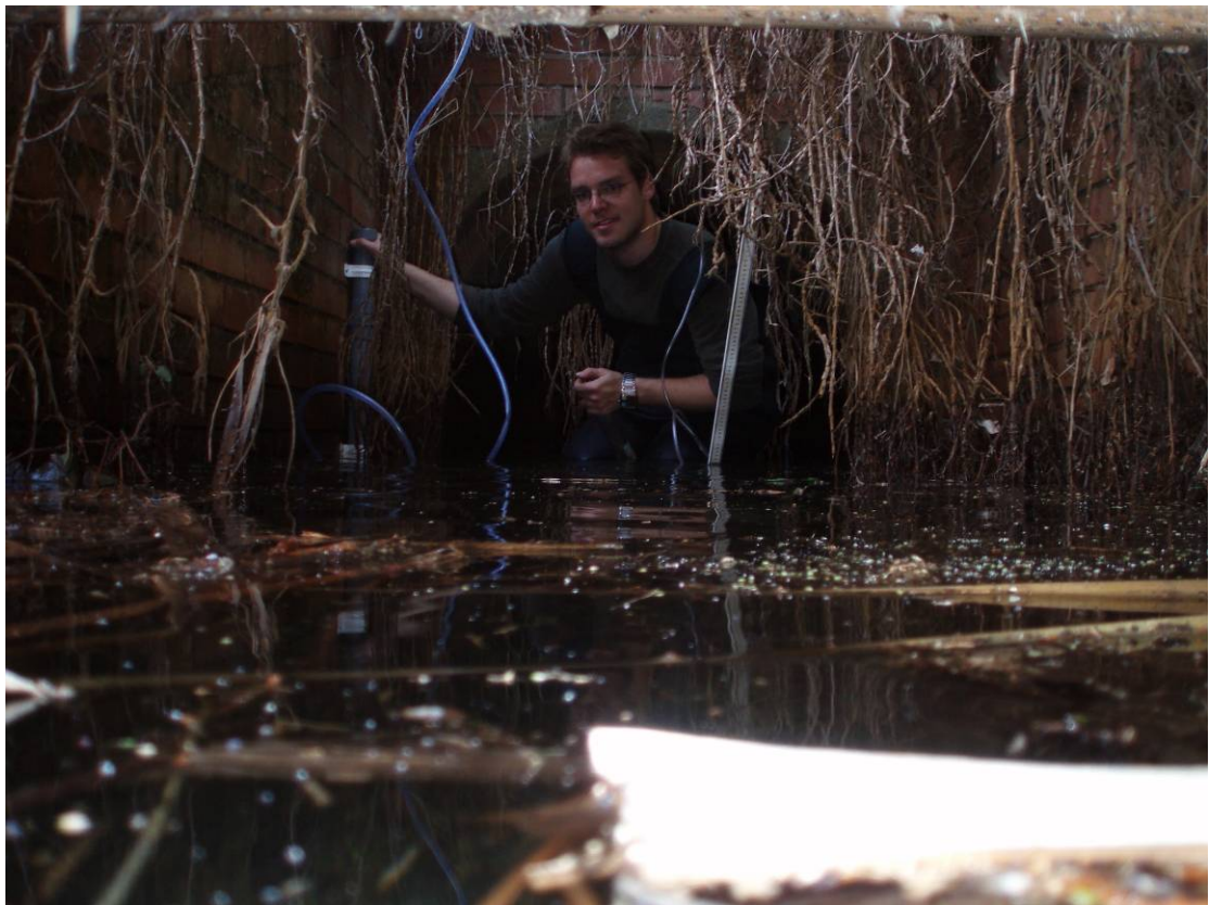
Figure 13: Installation of YSI Sonde unit in Brushfield Wetland output drain.
