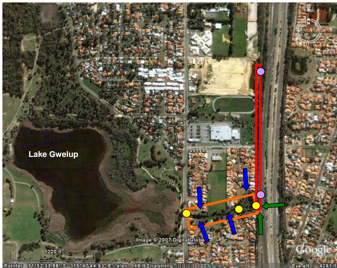
Figure 1: Aerial view of the Brushfield Wetland (orange outline), Delwaney Drain (red outline), two below-ground drains (green arrows) and four local roadway drains (blue arrows). Yellow circles represent the Brushfield Wetland monitoring sites (input, mid-point and output) and purple circles indicate Delwaney Drain monitoring sites (north and south).
