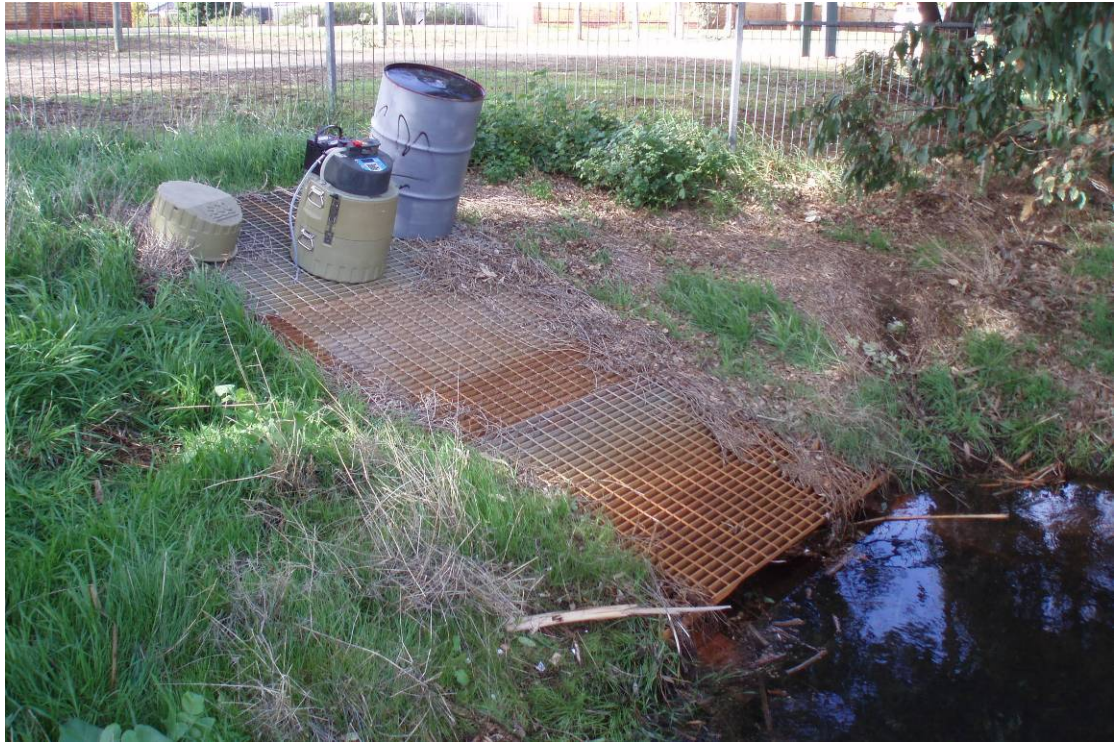
Figure 12: Brushfield Wetland output drain sampling site showing ISCO 6700 autosampler.
